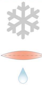
MELTED SNOW BY WARMING AIR IN ETFE
